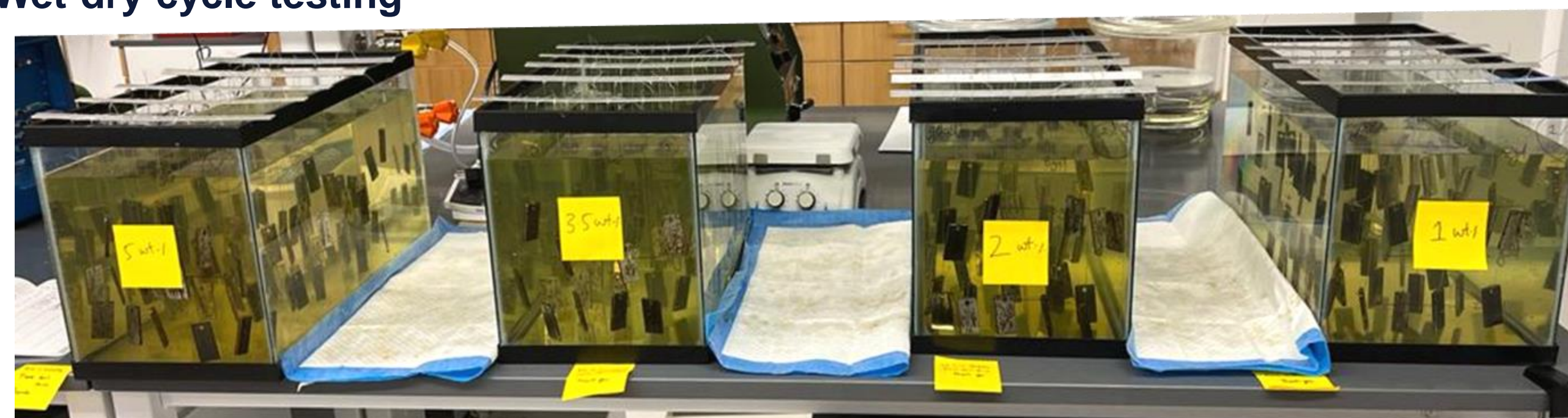
Fig. Wet-Dry cycle test setup
