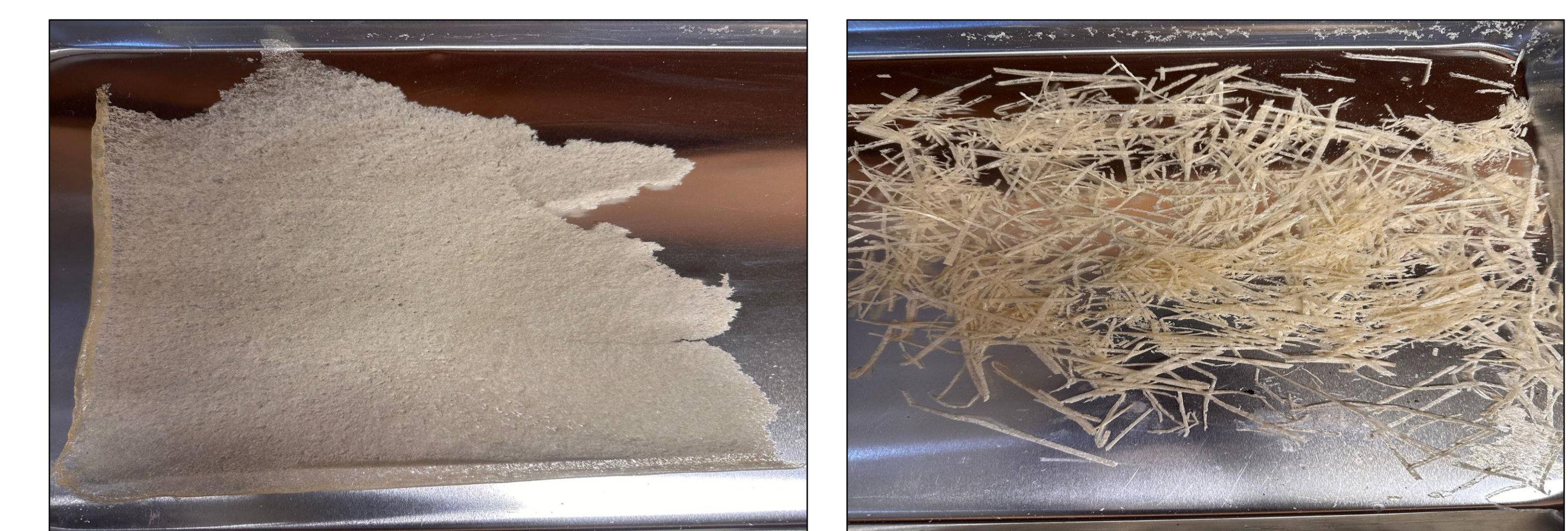
Figure 3. Newly prepared chitosan fiber sheet (left), chitosan fiber after being cut using a paper cutter (right)
