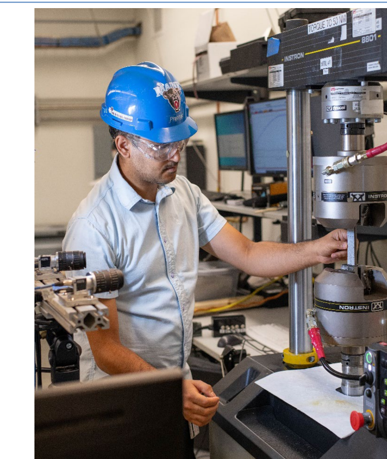
Figure 5: Conduction of Tensile Test to evaluate material properties.
