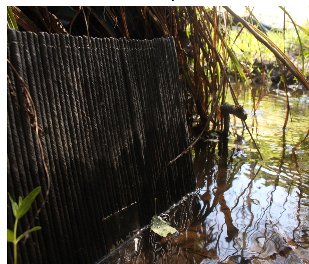
Figure 2: 3D printed witness panel installed at site for real exposure to moisture.
