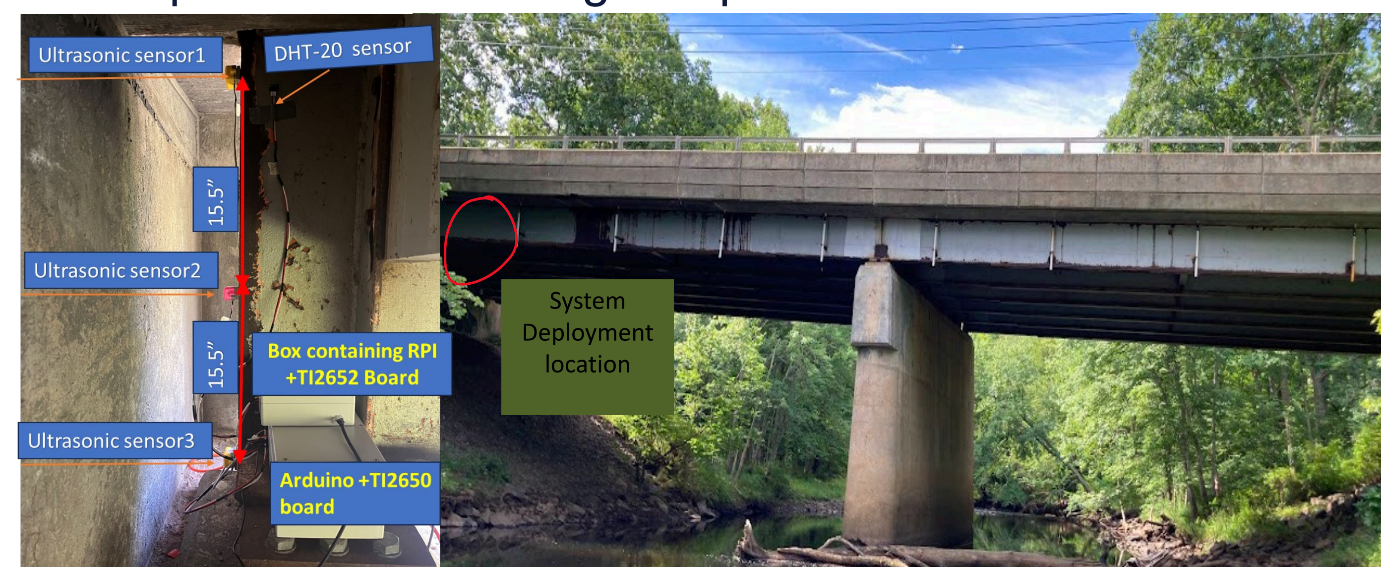
Testbed bridge with sensor location on the expansion gap and system
