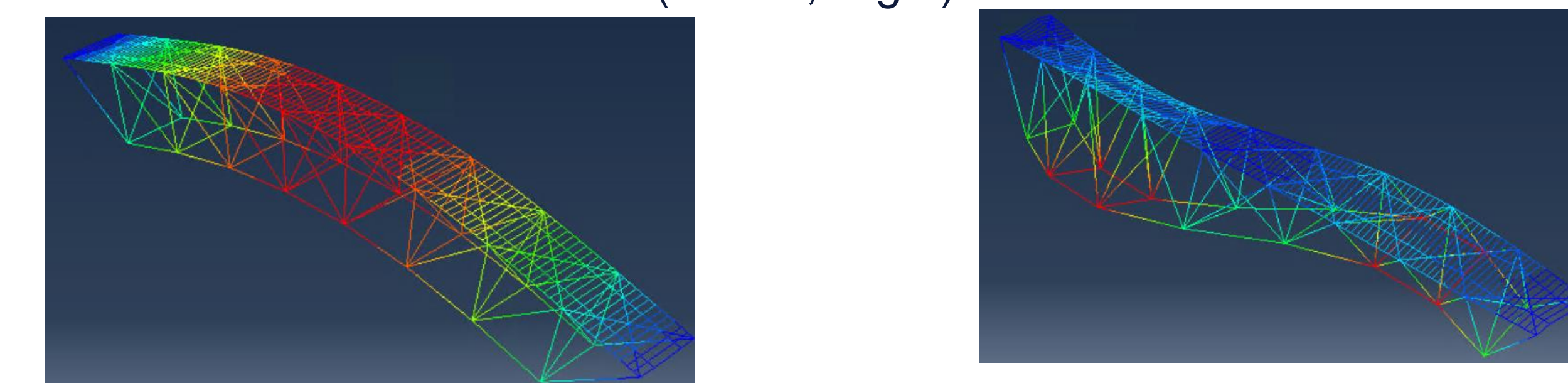
Fig. 5: First Vertical Mode Shape (1.2 Hz, Left); First Twisting Mode Shape (2.0 Hz, Right)
